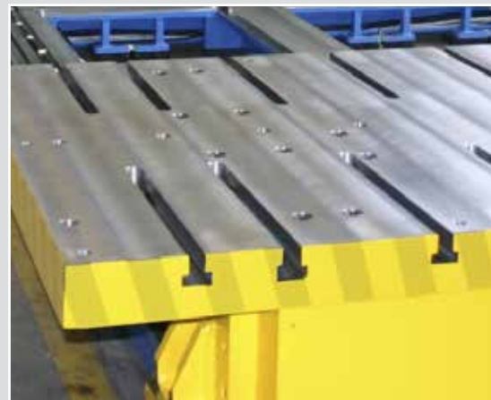
"T" slots on the whole surface.
