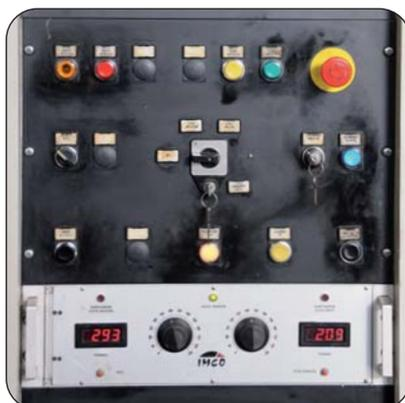
Load monitor integrated in the control cabinet
