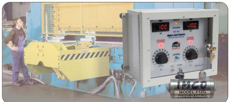
Overload monitor 2 digital dials and its "piezoelectric stress sensor"
