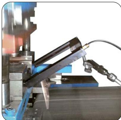
Frame sensor to check parts
