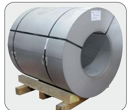
Large coils delivered with horizontal axis
